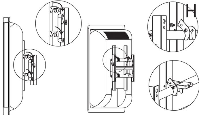
1. Hang the LCD TV assembled with the Bracket (D) on the Wall Mount (A) mounted on the wall.
