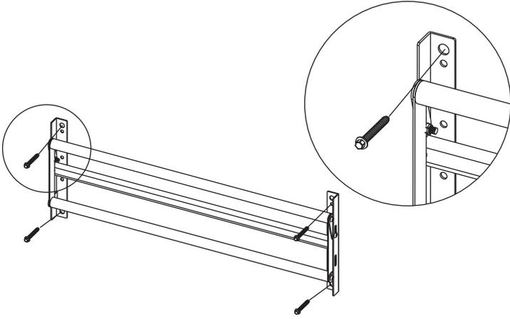
1. Wooden Wall or Drywall -drill a  $\varnothing 5.0$ mm pilot hole at each location using an electric drill. Fix Wall Mount(A) to the wall using the Hex Lag Bolts(B).
