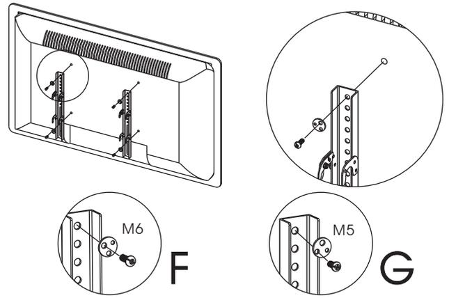
1. Take out screws F & G and choose the suitable screw which mostly match the VESA holes at the back of LCD TV. Then go through the matched hole on the Washer(E). (For example, if M6 screw is the matched screw, then it should go through the biggest hole on the washer(E).)
