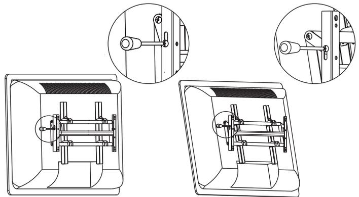
1. Use screw driver to loose the bolts at both sides.
